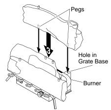
Figure 29 - Installing Rear Log (#3) (CCL3930NTA Shown)
